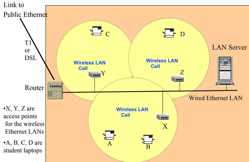
Figure 1-10: A Sample Configuration with Wireless Ethernet LANs
