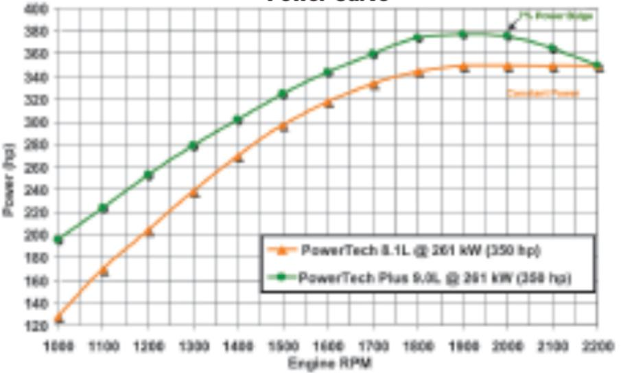
**Tier 3 PowerTech Plus 9.0L vs. Tier 2 PowerTech 8.1L**
