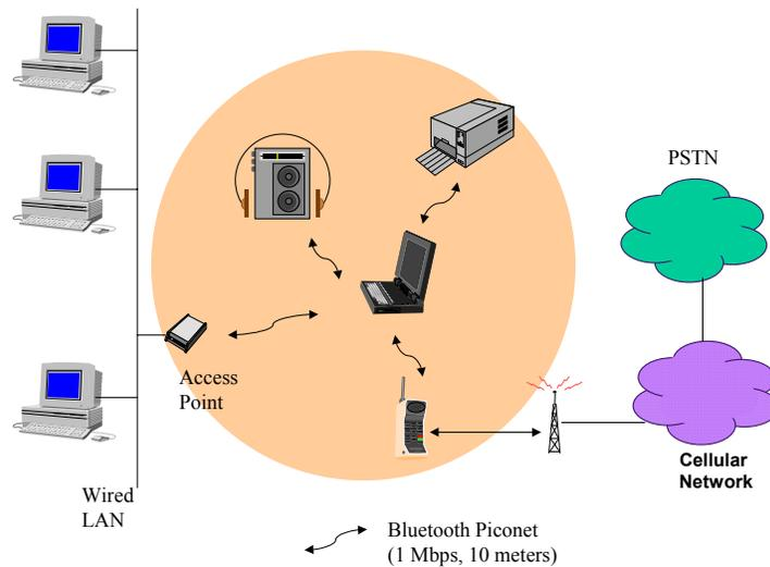
Figure 1-11: A Simple Bluetooth Configuration
