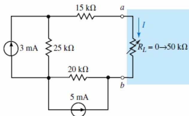
33. a.  $I_N = 0.417 \text{ mA}$ ,  $R_N = 60 \text{ k}\Omega$
