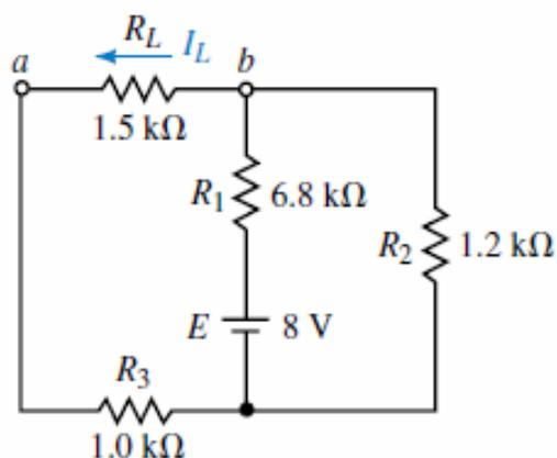
$$27. I_N = 0.594\text{ mA}, \quad R_N = 2.02\text{ k}\Omega, \quad I_L = 0.341\text{ mA}$$
