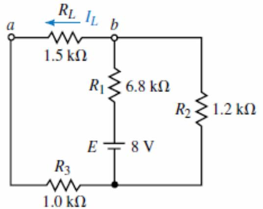
$$9. R_{Th} = 2.02 \text{ k}\Omega \quad E_{Th} = 1.20 \text{ V} \quad V_{ab} = -0.511 \text{ V}$$
